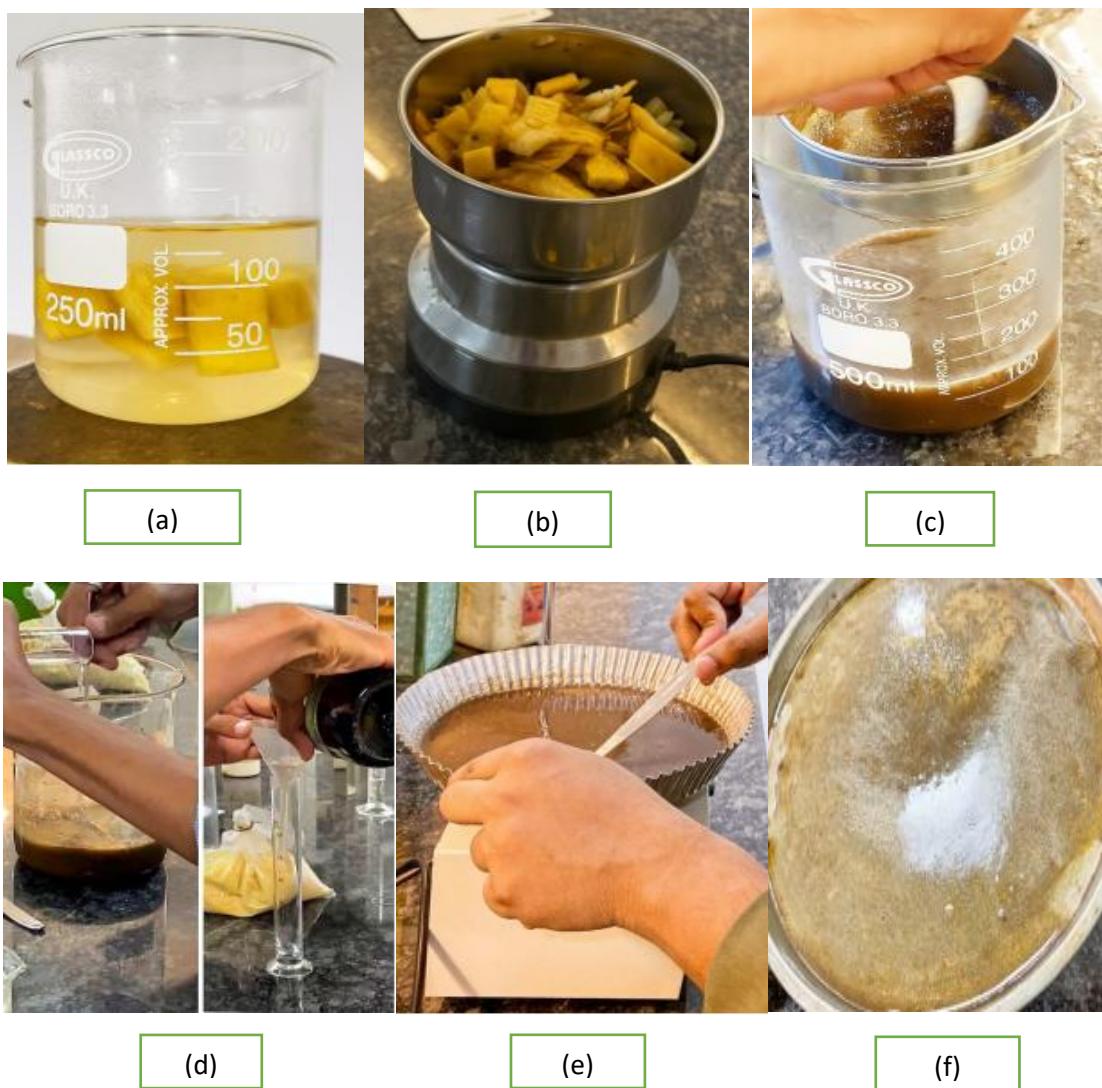
Figure 3. Stepwise preparation of biodegradable plastic film from banana peels
